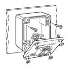
(8) Reassemble the switch box with the 4 screws.
