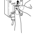
4 Push and hold [PTT], then transmit the appropriate information (vessel's name, your position, nature of the distress, assistance required, etc.)
